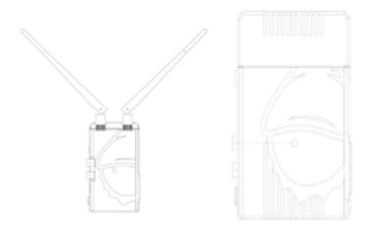
Position the antennas on the transmitter and receiver at right angles as shown in the illustration. This ensures the best possible RF performance.
