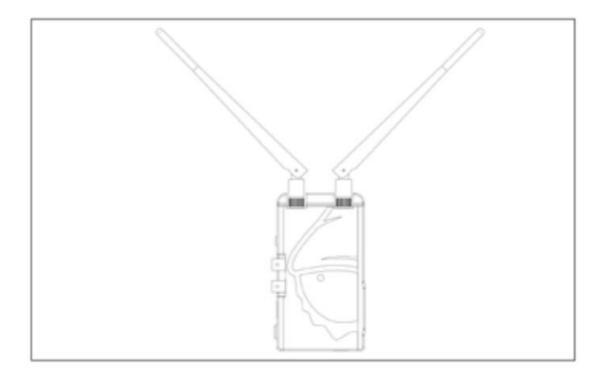
Position the antennas on transmitter and receiver as shown in the illustration.
