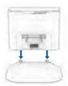
Place the charging station on a hard, flat surface, away from edges & stairs, with plenty of room around it. Plug it into the outlet.
