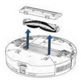
4. Clean the main brush and all its components, including the brush gate and brush compartment.
