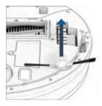
2. Remove debris from the side brush and its socket.
