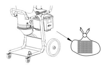
Close the bag using the supplied cable ties when you believe that it has been filled to a suitable level. Another cable tie is used a little further up. This forms the bottom of the next bag. The filled bag is then cut off, and the machine is ready to be used again.
