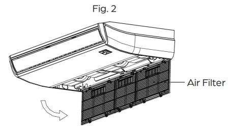
3. Remove the air filter. (Fig. 3)
