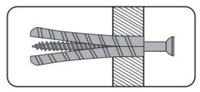
Generally aerated blocks should not be used to support heavy loads, use a specialist fitting in this case. For light loads, a General Purpose Plug can be used.
