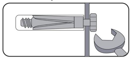
For use with walls stuck with plaster board. The hammer fixed allows it to be fixed to the wall rather than the plaster board. Always check the fixed is secure to the retaining wall.
