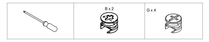
WHEN FITTING CAMS ENSURE STARTING POSITION IS CORRECT BEFORE YOU INSERT CONNECTING CAM-PILLAR TURN CLOCKWISE UNTIL SECURE
