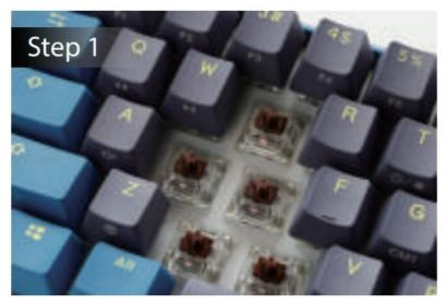
2. Use switch puller to pull out the switches.
