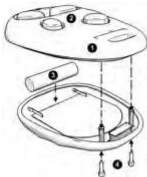
■ Remote control PULT 6204 powered by one 27A 12V battery
