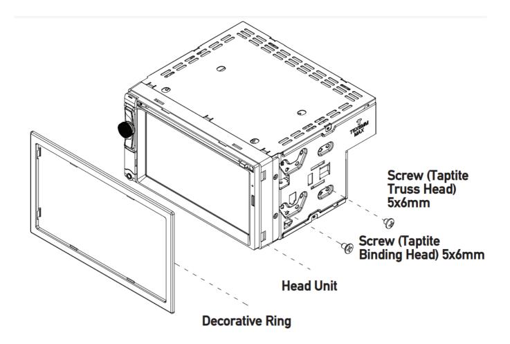
TYPICAL FRONT-LOAD MOUNTING METHOD
