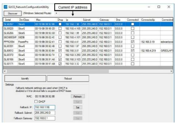
Note: Clicking on Identify for any selected device will cause the unit's LED to flash.
