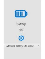
The drop-down menu allows users to quickly switch the power modes of the tablet. S elect Max Battery Performance Mode to enable the system performance, and to sa ve the system power, select Extended Battery Life Mode.
