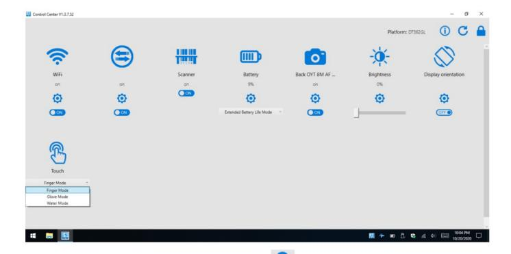
To access the Authorized User Mode, click on the lock icon on the top right corner of the application window, then a dialogue window opens for the authorized user to enter the password. The default password is P@ssw0rd.
