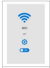
Tap the On/Off button to enable or disable the WLAN connection.\*
