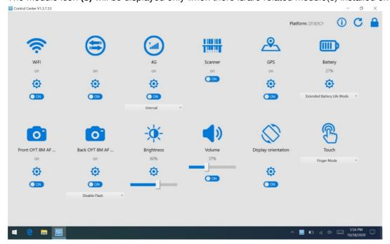
To access the **Authorized User Mode**, click on the lock icon on the top right corner of the application window, then a dialogue window opens for the authorized user to enter the password. The default password is **P@ssw0rd**.
