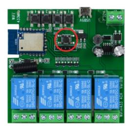
In the center of the board is the reset button. If you hold down the reset button for 5 seconds restore factory settings and the device goes into standby mode app setup with the blue LED flashing quickly.
