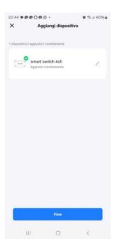
Now the device is connected to the wifi network. If the wifi connection is lost, the device will automatically activate the Bluetooth connection.
