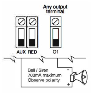
**NOTE:** The PC5204 is not suitable for fire alarm annunciation.
