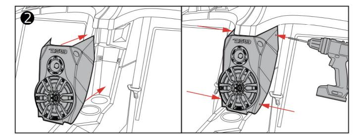
Then secure the pod (Picture 4) and reconnect the 12V port in the new hole position and re-connect it. (Picture 3)
