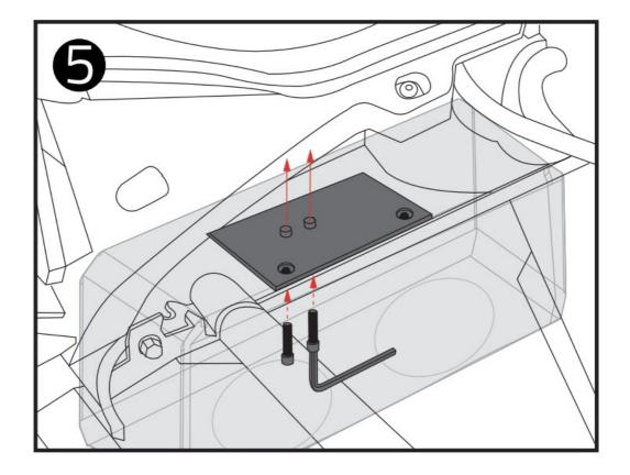
Do not forget to put back the damping material and install back the Subwoofers, be careful not to over-tighten or the hole may be damaged and not properly secure the subwoofer. (Picture 6)
