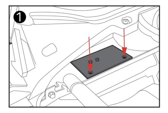
For the pass-through screws, if you have a 2017-Up all the holes are pre-drilled from factory, for older model you need to open these two holes using a  $\frac{1}{2}$ " drill bit. (Picture 2)
