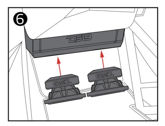
This kit needs an aftermarket amp pre-installed with the speaker wires in this location, only after this step can you install the speakers using the aftermarket amp's speaker wire.
