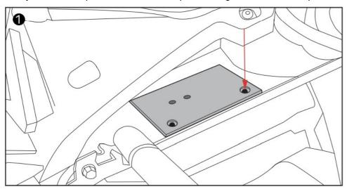
2. For the pass-through screws, if you have a model from 2017 or later all the holes are pre-drilled from factory, for older models you need to open these two holes using a ½" drill bit. (**Picture 2**)
