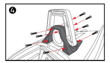
Re-install the rear hoop accent in the same way that factory was pulled out. (Picture 4) This concludes the passenger side installation of the SLG-HD6 pod, then move next to the driver side.
