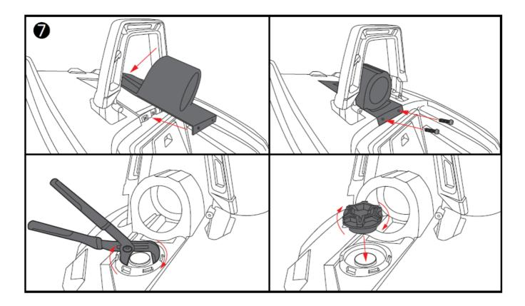
Now, carefully slide in the new speaker pod in place and secure it using the factory T25 bolts on front bottom of the piece, then re-install the Ring-Nut and the gas cap. (Picture 7)
