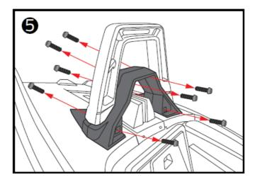
Remove the factory rear hoop accent using a T40 TORX socket to extract the (2) screws on bottom of the piece and a T25 TORX to extract the (2) screws on top of the piece and pull it to the front, then using the T40 TORX to extract the (2) screws in the back of the piece and pull it to the back. (Picture 5)
