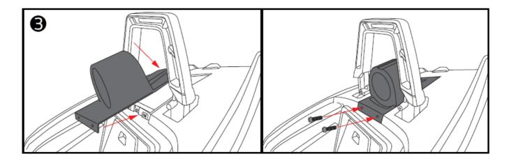
Install the new speaker pod in the same way that factory was pulled out and secure it using the factory T25 bolts on front bottom of the piece. (Picture 3)
