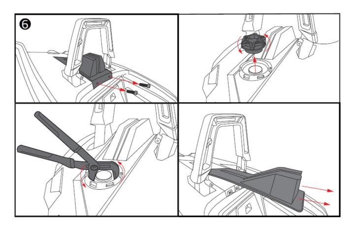
Remove the factory rear deck hump using a T25 TORX socket to extract the (2) screws on front bottom of the piece, then remove the gas cap and using an oversized pliers, un-screw the Ring-Nut that holds the gas tube in place, after this you can pull out the piece. (Picture 6)
