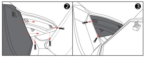
3. Remove the factory panel and install the new SLG-AR6 Pods the same way that factory was pulled out. (Picture 4) (Picture 5)
