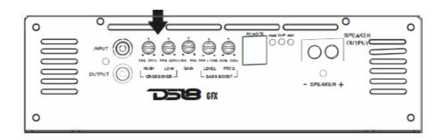
D518 GFX amps amplifiers have an adjustable bass boost. Begin your adjustments at low volume. If you do not hear any improvement then woofer does not need any bass boost. Use Bass Boost carefully. The demands on power output are tremendous. Try to minimize the use by changing woofer position or the enclosure size.
