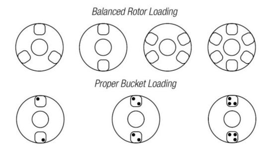
Buckets can be placed around the rotor in any of the rotor loading configurations shown. Each bucket must be loaded symmetrically with tubes as above.
