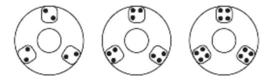
When all six buckets are being used, the rotor must be loaded in the following configuration only. Opposing buckets do not need to be filled but must be loaded in exactly the same way.
