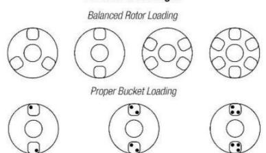
Buckets can be placed around the rotor in any of the rotor loading configurations shown. Each bucket must be loaded symmetrically with tubes as above.
