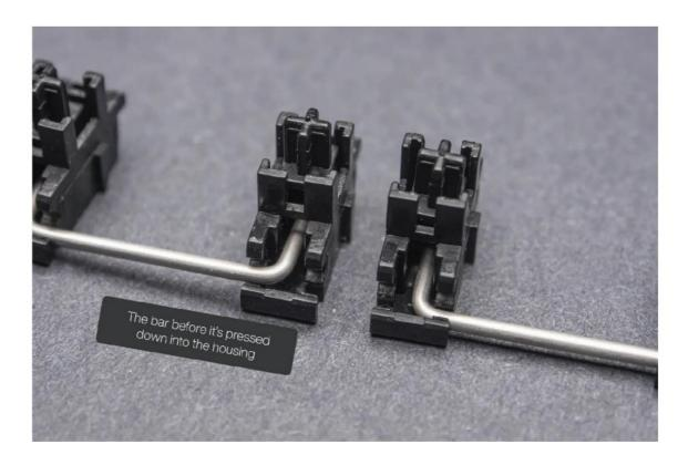
Repeat the same process for the other side. Repeat for all stabilizers. Below is an image of an assembled stabilizer.
