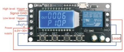
Wiring diagram for sharing one power supply
