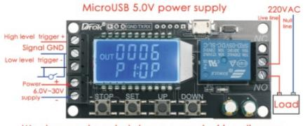
Weak current control strong current wiring diagram
