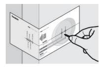
C. Mark hole on the edge of the door. Select door thickness before marking hole.
