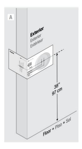
A. Select the template that allows you to place the template on the EXTERIOR side of the door. Fold template along fold line and place fold line along the edge of the door. Place centerline approximately 38" (97 cm) from the door.
