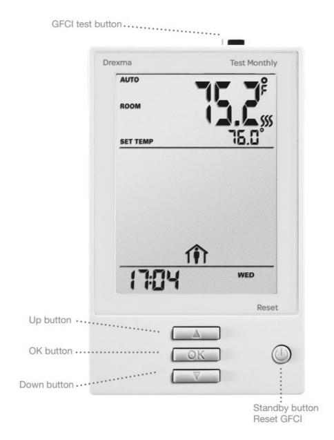
Adjust the setpoint until the heating symbol ( ) appears. Use the Up button to increase the heating demand and then press the OK button
