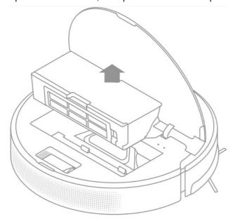
2. Open the bin cover and empty the bin as shown in the diagram.
