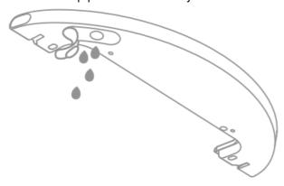
3. Pour out the water in the tank. Clean with only water and leave out to air dry before re-installing. **Note:** Do not expose the tank to the sun directly.
