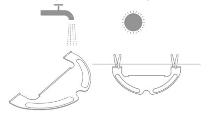
4. If slow water flow occurs, or the volume is not well-distributed, clean the airhole in the cover of the water tank.
