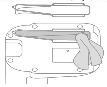
3. Reinstall the air duct cover as shown in the diagram.
