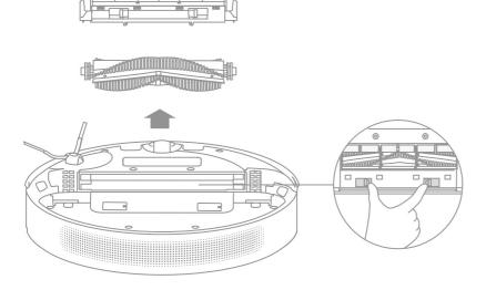
Pull out the brush covers as shown in the diagram. Use the included cleaning tool to remove any hairs tangled in the brush.
