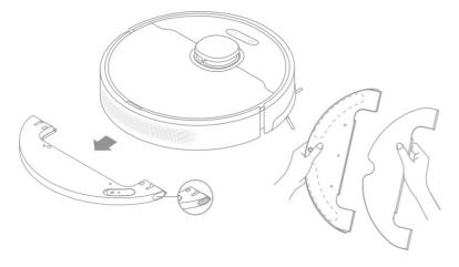
2. Clean the mop pad with water only and leave to air dry before re-installing.
