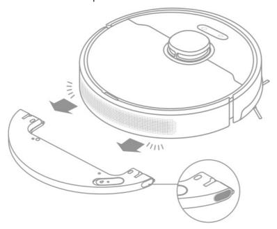
**Note**: When the robot is charging or not in use, remove the mopping module, pour out all the remaining water in the tank, and clean the mop pad to prevent mildew or odors.
