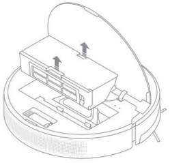
2. Open the dust box cover and empty the dust box as shown in the diagram.
