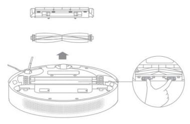
2. Pull out the brush covers at both ends of the brush as shown in the diagram. Use the provided cleaning tool to remove any hairs tangled in the brush. Reinstall the brush covers on both ends of the brush, and then reinstall the brush. Press on the brush guard to lock it in place.
