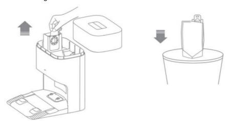
**Note:** Pulling outwards on the handle will seal the dust bag to prevent the dust and debris from accidentally falling out.
