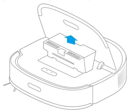
2. Open the bin cover and empty the bin as shown in the diagram.
