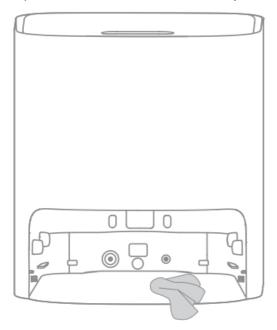
4. Insert the washboard into the base as shown in the diagram, making sure that both clips are in place.
