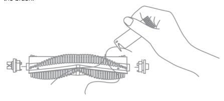
Note: Do not pull out the hair tangled in the brush excessively. Otherwise, the main brush may be damaged.
