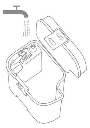
**Note:** The floating ball in the waste tank is a moving part. Do not clean the floating ball excessively in case of affecting its functions.
