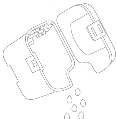
2. Clean the waste tank with water and put it back to the base.
