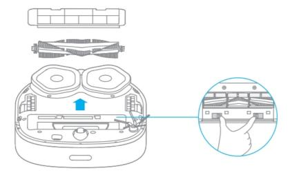
Pull out the brush covers as shown in the diagram. Use the provided cleaning tool to remove the hair tangled in the brush.
