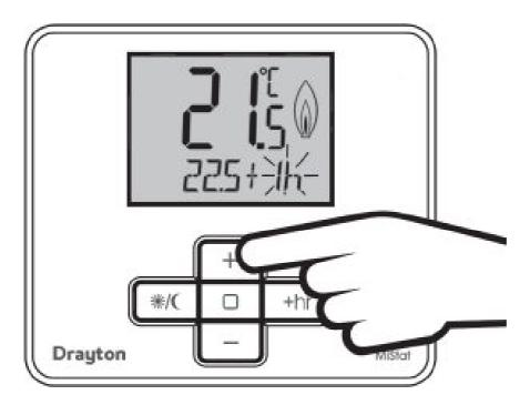
Press +/- to adjust +hr period between 0 and 3 hours Press (□) to confirm Now the Boost is running. The time will be counted down each hour. Once the time has elapsed, control returns to the prior temperature screen. The Boost can be cancelled by pressing the (☀/) key or by setting the +hr period to 0.
