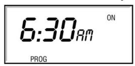
• Press SET?, and you'll see OFF1, the end of your first heating period. Adjust this in the same way, press SET?, then repeat the procedure for ON2, OFF2, ON3 and OFF3.
