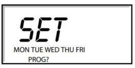
• When you press SET? after OFF3 for SAT SUN, the timeswitch will return to normal operation.
