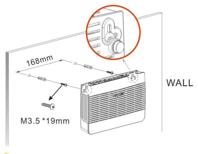
**Note** The recommended drill diameter shall be 6.5mm (1/4).
