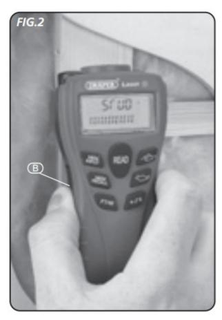
Place the detector flat against the wall. Press and hold button to calibrate the unit. The buzzer will sound to confirm and the display will read 'Stud'.
