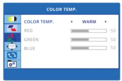
**COLOR TEMPERATURE:** Select the color temperature from the pre-set "Warm" or "Cool", or select "User". Users can set the color temperature under the User setting mode by adjusting the red, green and blue parameters.
