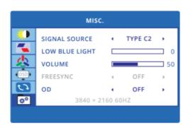
**SIGNAL SOURCE:** Select the video signal from HDMI port, USB-C 1 and USB-C 2.
