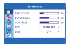
**BRIGHTNESS:** Adjust the brightness parameter of the image. The adjusting range is from 0 to 100. The default setting is "20".
