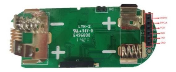
USB to TTL <- -> LWL02 RX <- -> TX TX <- -> RX GND <- -> GND
