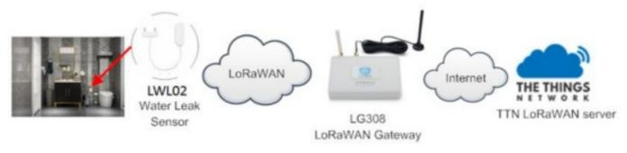
The LWL02 has water leak detect probe as above. When there is water between these two detect probe, they will be short and generate the water leak event. and send the status to LoRaWAN server.
