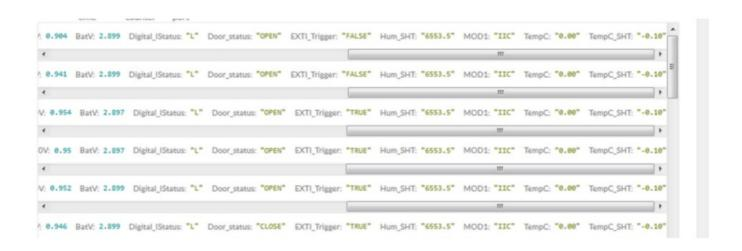
In MOD:1, the user can use byte 6 to see the status of the door open or closing. TTN V3 decoder is as below: door= (bytes[6] & 0x80)? "CLOSE":"OPEN";
