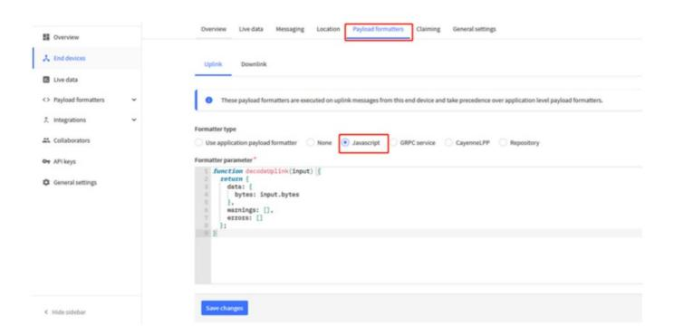
**The payload decoder function for TTN V3 are here:** SN50v3-LB TTN V3 Payload Decoder: <a href="https://github.com/dragino/dragino-end-node-decoder">https://github.com/dragino/dragino-end-node-decoder</a>
