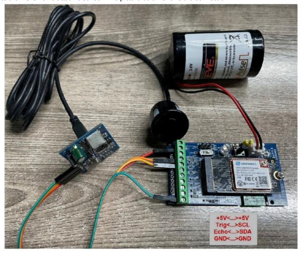
Connect to the SN50v3-LB and run AT +MOD:2 to switch to ultrasonic mode (ULT). The ultrasonic sensor uses the 8th and 9th byte for the measurement value.
