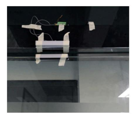
The above photos shows the two parts of the magnetic switch fitted to a door. The software by default uses the falling edge on the signal line as an interrupt. We need to modify it to accept both the rising edge ( $0v \rightarrow VCC$ , door close) and the falling edge ( $VCC \rightarrow 0v$ , door open) as the interrupt. The command is:
