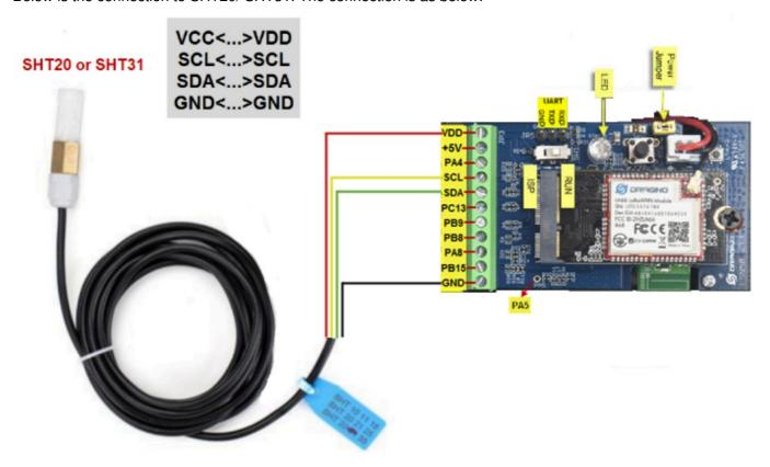
The device will be able to get the I2C sensor data now and upload it to the IoT Server.
