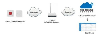
**Step 1:** Create a device in TTN V3 with the OTAA keys from PB01. Each PB01 is shipped with a sticker with the default DEV EUI as below:
