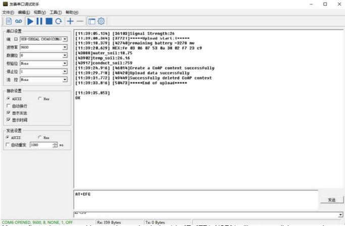
After configure the server address and reset the device (via AT+ATZ), NSE01 will start to uplink sensor values to CoAP server.
