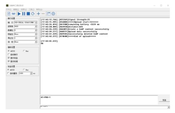
After configure the server address and reset the device (via AT+ATZ), NDDS75 will start to uplink sensor values to CoAP server.
