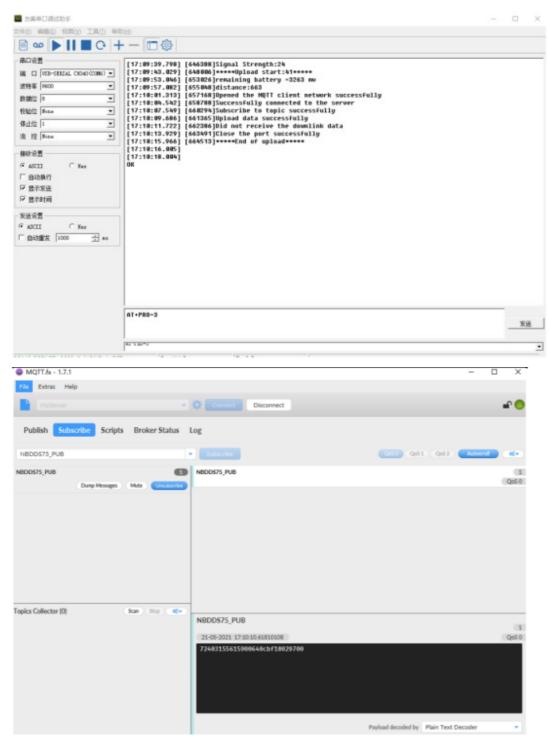
MQTT protocol has a much higher power consumption compare vs UDP / CoAP protocol. Please check the power analyze document and adjust the uplink period to a suitable interval.
