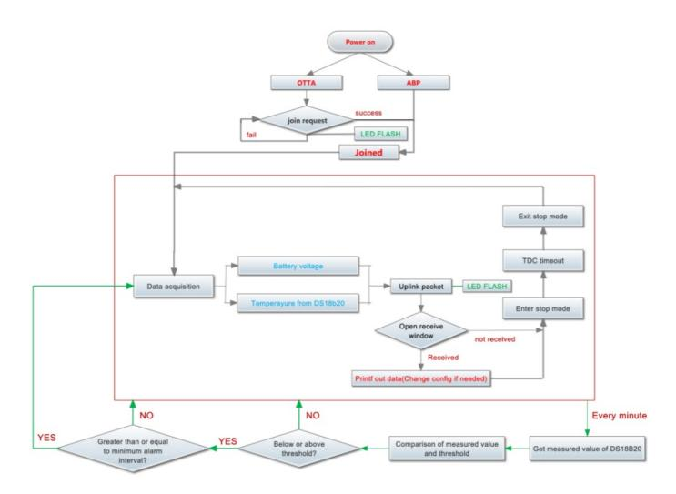
User can use AT+18ALARM command to set the alarm low limit or high limit. Device will check the temperature every minute, if the temperature lower than low limit or greater than high limit. LSN50v2-D2x will send an Alarm packet base on Confirmed Uplink Mode to server.
