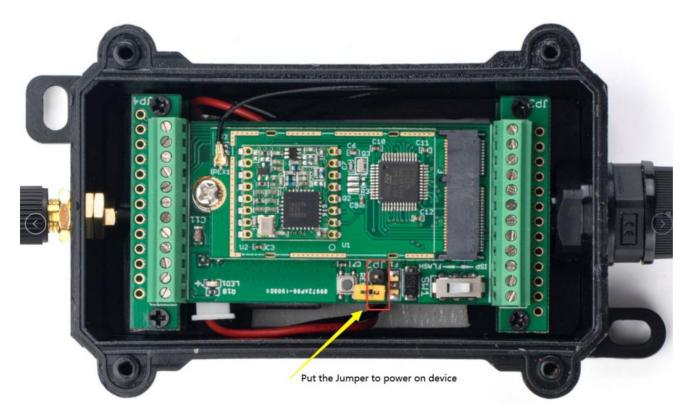
• Step 3: LSN50V2-D20 will auto join to TTN network via the LoRaWAN coverage by DLOS8. After join success, LSN50V2-D20 will start to uplink temperature value to server.
