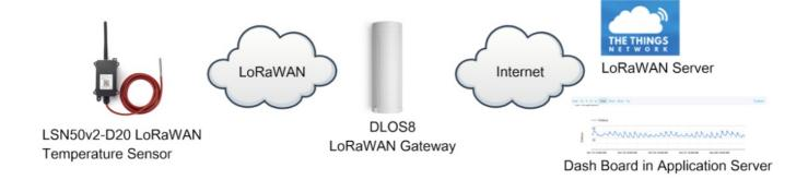
LSN50V2-D2x LoRaWAN Waterproof, Outdoor Temperature Sensor
