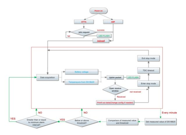
User can use AT+18ALARM command to set the alarm low limit or high limit. Device will check the temperature every minute, if the temperature lower than low limit or greater than high limit. LSN50v2-D20 will send an Alarm packet base on Confirmed Uplink Mode to server.
