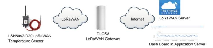
The DLOS8 is already set to connect to <a href="ITN">ITN</a>. What the rest we need to is register the LSN50V2-D20 to TTN: **Step 1:** Create a device in TTN with the OTAA keys from LSN50V2-D20. Each LSN50V2-D20 is shipped with a sticker with the default device EUI as below:
