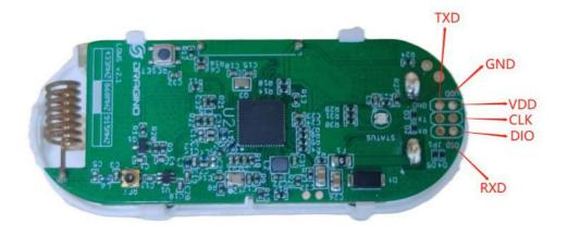
USB to TTL <- -> LDS02 RX <- -> TXD TX <- -> RXD GND <- -> GND
