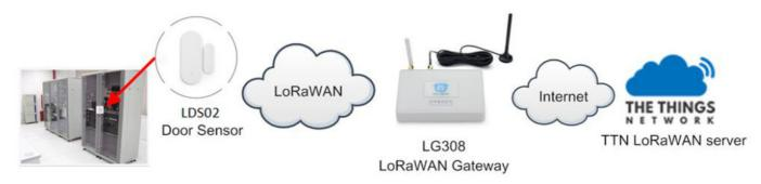
The LDS02 in installed on the door edge to detect the open / close event. And send the status to LoRaWAN server. The LDS02 will uplink two type of messages to the server.
