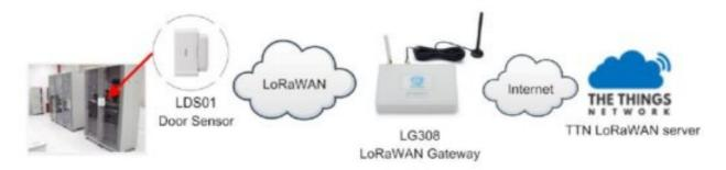
The LDS01 in installed on the door edge to detect the open/close event. And send the status to the LoRaWAN server. The LDS01 will uplink two type of messages to the server.
