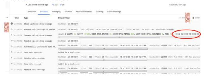
Example Payload Decoder in TTN V3: <a href="http://www.dragino.com">http://www.dragino.com</a>/downloads/index.php? dir=LoRa\_End\_Node/LDS01/Payload/
