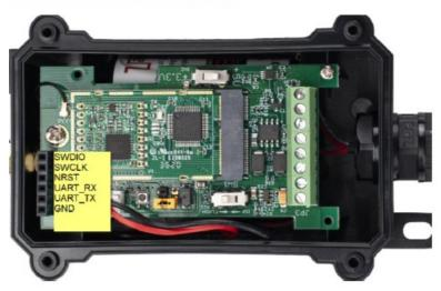
In the PC, you need to set the serial baud rate to 9600 to access the serial console for LDDS75. LDDS75 will output system info once power on as below:
