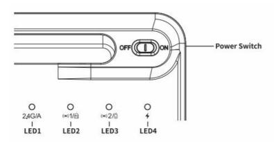
**Power On/Off:** Toggle the switch to ON. The blue indicator will be on and then off after 5 seconds, indicating the keyboard has been powered on. Toggle the switch to OFF to turn off the keyboard.
