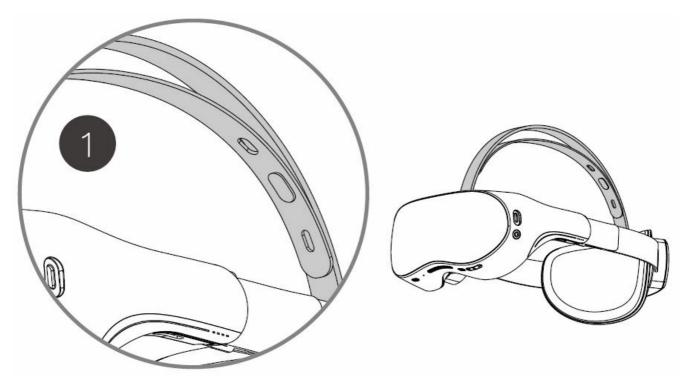
3. The side head strap passes through the slots on both sides of the headset. Loop the straps through the slots and adjust to a suitable position.
