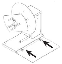
2. Load the empty cardboard core, let pass the printed media underneath the tension arm and stick it on the core. Slide in the outer disk onto the core holder and keep it close to the media edge. Once the media is loaded on the rewinder, slide left and right the rewinder to find the correct alignment with the printer.
