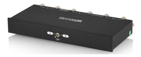
SP102 is a passive audio selector, convenient to compare the sound quality of 2 pair of different speakers or 2PCS amplifiers. Each channel can pass through power up to 200W, fully isolated design for all channels and the GND of each channel is independent, also with built-in protective loads for channels A&B, suitable for all types of amplifiers. Proper size with simple appearance, fashionable and durable, convenient for use in most situations.
